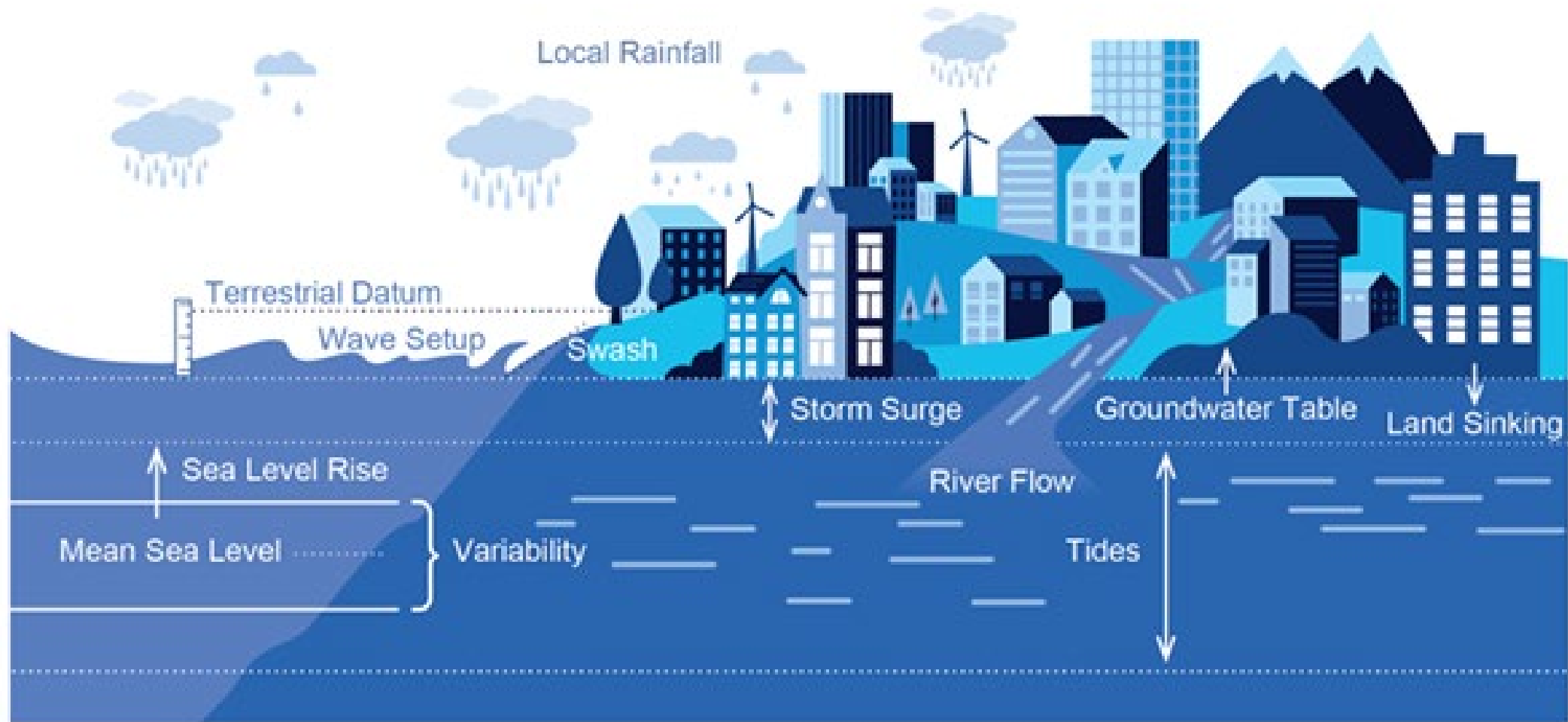
Figure 1.1: Schematic (not to scale) showing physical factors affecting coastal flood exposure. Due to the clear and strong relative sea level rise signal (i.e., combination of sea level rise and sinking lands), the probability of flooding and impacts are increasing along most U.S. coastlines.
